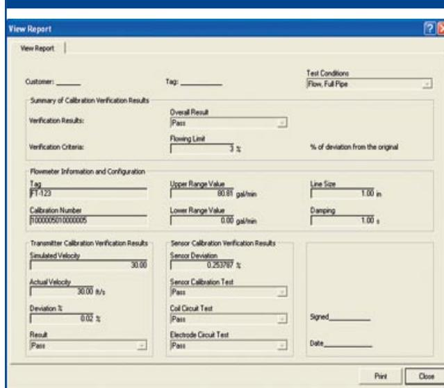
values or charts that need interpretation, but rather offers clear, actionable information. If the result is “fail”, the technician schedules calibration, or if damaged, replaces the flow sensor. If the result is “pass”, calibration can wait.
