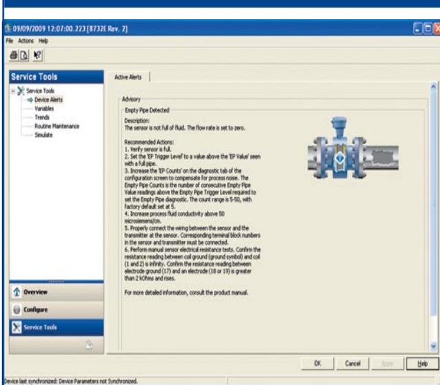
enabling corrective action to be taken sooner. EDDL is used by the magnetic flowmeter manufacturer's expert to share know-how in the form of text and illustrations which guide the technician toward a resolution for the problem.
