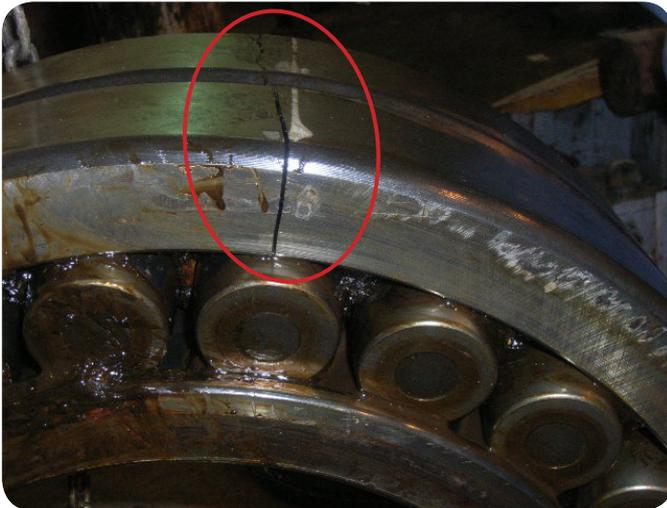
Analysis proved to be correct when the bearing was removed and inspected. The outer race was cracked, and flaking had begun
