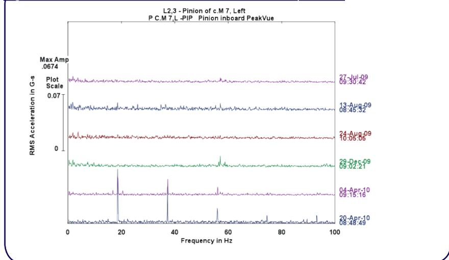
unusual. Then, additional PeakVue measurements made on April 20 revealed a big change. The five very apparent spikes in Figure 1 were the earliest indication of a serious problem. This is the story of using Emerson's PeakVue technology to make predictions of the bearing's expected run-life, which led to an order to stop the mill for repairs. In this case, the downtime was limited to about 12 hours to replace the faulty bearing.
