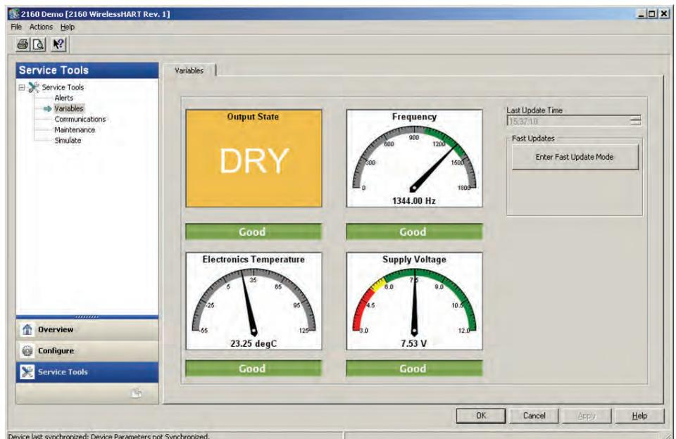
Device details such as frequency and power module status facilitate troubleshooting.
