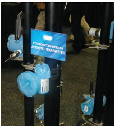
*In steam trap monitoring, a wireless acoustic transmitter 'listens' for ultrasonic noise created by steam or condensate, and also measures the temperature at the steam trap inlet via a built-in sensor.*
