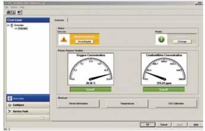
NE107 defines standard icons and colors to signal the device status, which makes assessment of device health easier.
