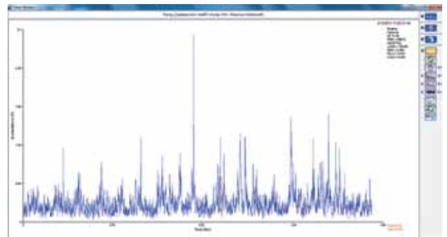
*Specialised machinery health monitoring software in the reliability office enables analysis of vibration in equipment such as motors and pumps around the plant.*
