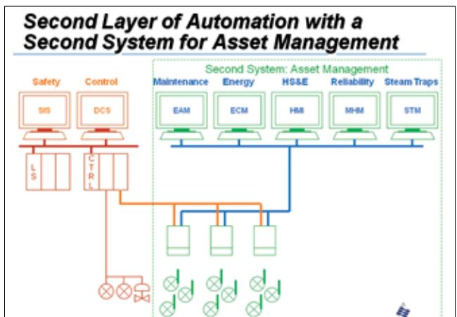
Data from WirelessHART transmitters go to the control system and the asset management system.
