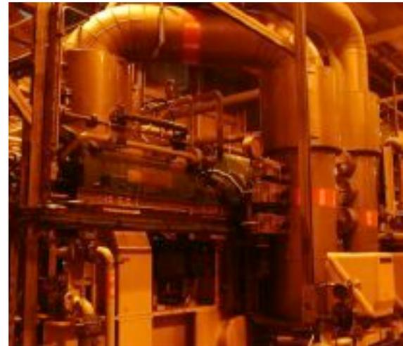
Figure 2 Gas compressor on the Shell Draugen platform (Photo: Emerson Process Management)
