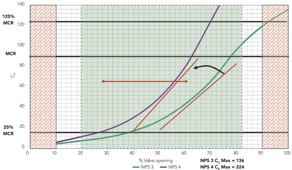
Figure 1. Oversized valve (NPS 4) can't provide adequate performance.
