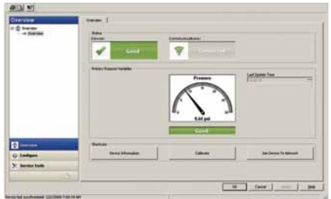
Thanks to EDDL, 4-20 mA, Foundation fieldbus, and WirelessHart have similar user interfaces, which makes it easy to manage a mix of devices.
