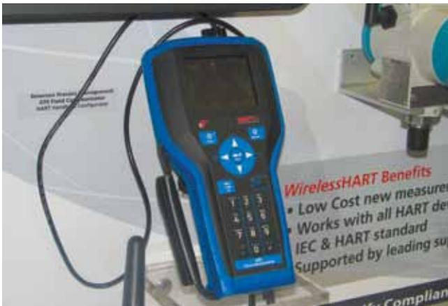
Handheld field communicators for 4-20 mA and Foundation fieldbus also work for WirelessHart.
