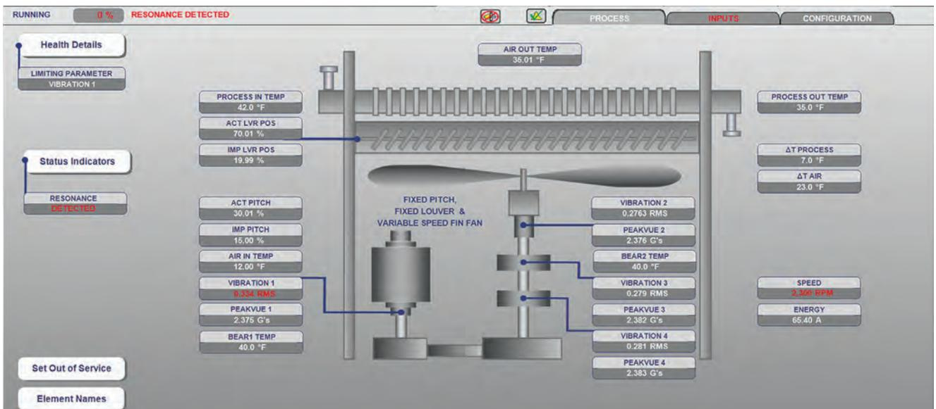
Figure 4: ACHE display – resonance alarm.
