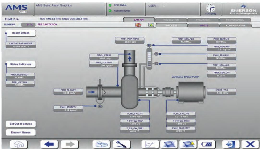
Figure 5: Pump display – pressure instability alarm.
