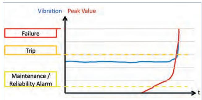
Figure 3: Alarming on peak value acceleration gives an even earlier warning of onset bearing defect.
