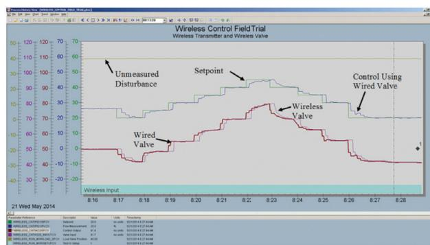
Figure 3: Setpoint change response, wireless transmitter and wired valve.
