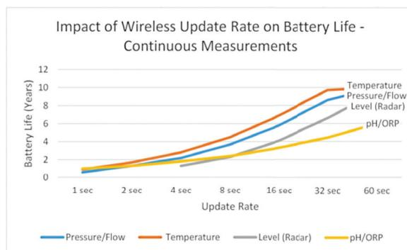
Figure 1: Impact of update rate on battery life
