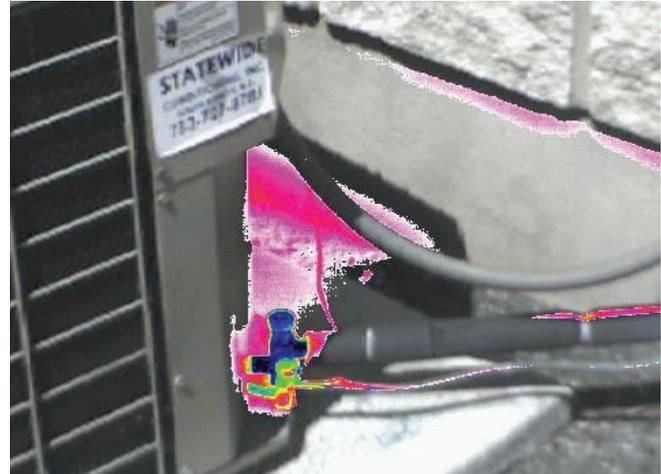
*The CSI 9830 Image Overlay Mode reveals the infrared data together with the visible image.*
