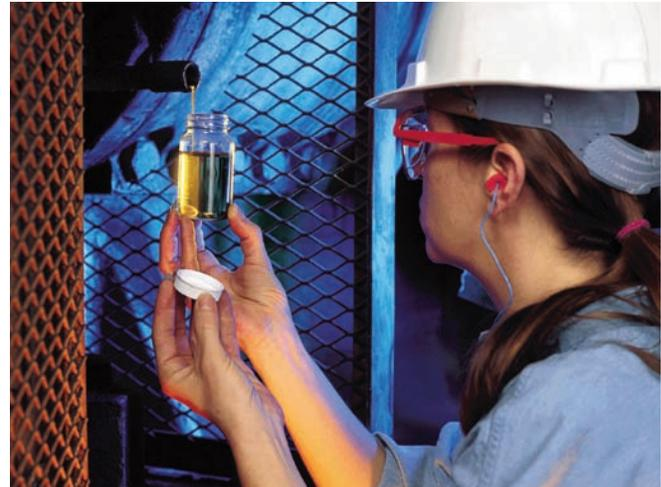
*Oil analysis data can be integrated with your vibration, infrared thermography, laser alignment and balancing data for a complete look at your machinery health.*
