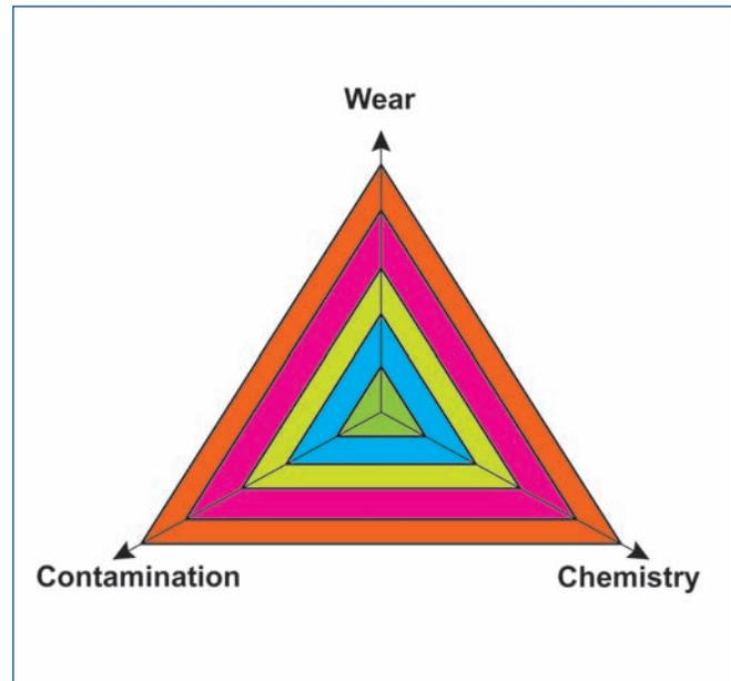
*Trivector examines three essential elements that determine oil and machinery condition.*
