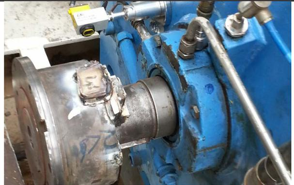
***“Using the CSI 2130, the team balanced a motor in place and returned it to normal vibration levels in less than a day – a feat that would have required up to three days if the motor was removed.”***
