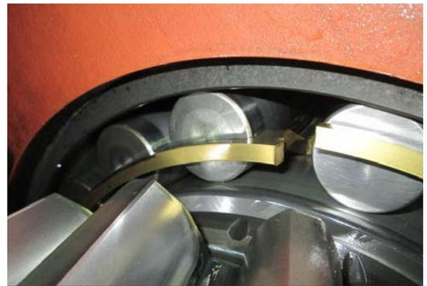
*Emerson’s Online Machinery Health Monitoring solution monitored the condition of a fracture in the gearbox’s bearings’ cage allowing safe production for 17 days.*
