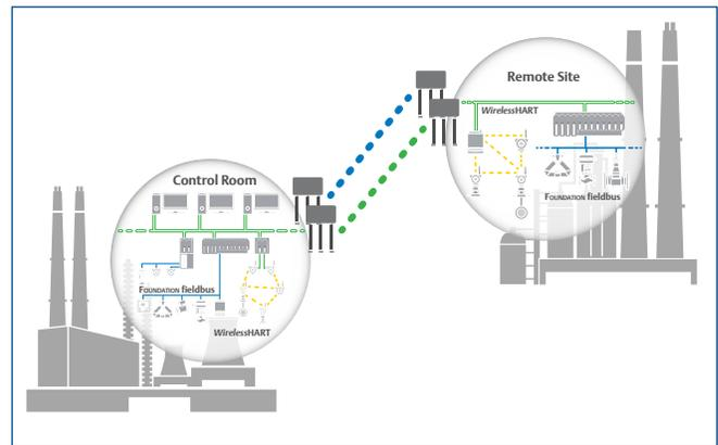
*An Emerson Smart Wireless Bridge Solution allows you to wirelessly extend your DeltaV™ Area Control Network.*
