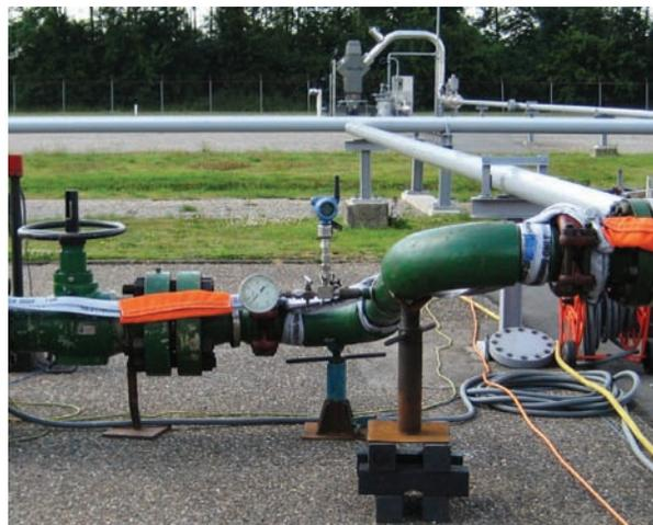
*Emerson’s wireless sensors are used by NAM to measure differential pressure and temperature as part of a mobile well head test system.*
