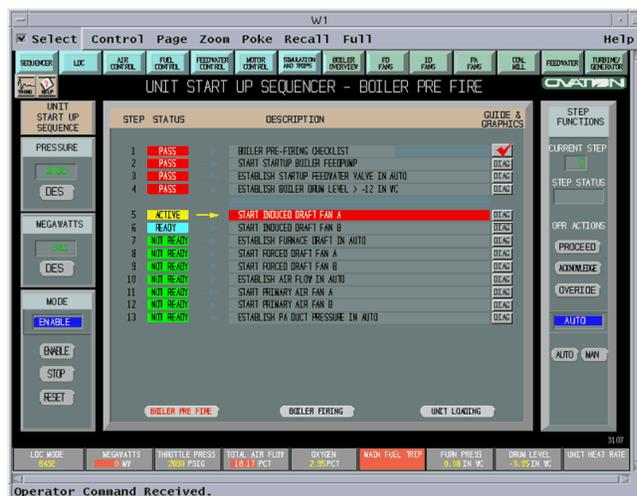
Automating startup can also eliminate human errors that can cause equipment damage and downtime. In effect, it's like having your best and most experienced operator running the startup -- every time.
