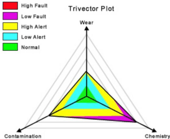
Lube oil analysis Tri-vector Plot combines contamination, oil chemistry, and wear analysis in a single severity plot. This sample shows water contamination and oil chemistry problems. Lubricant change is recommended.
