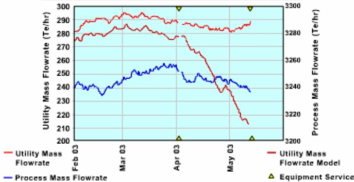
This graph shows increase in **utility** use while **throughput** and **heat** drop. Trending this allows you to predict when the unit will become heat-limited, allowing the unit to stay in operation until maintenance is absolutely required.
