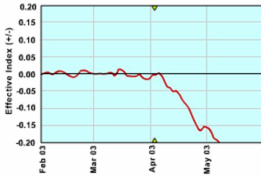
This graph shows heat exchanger efficiency dropping significantly. This drop may lead the process to become heat-limited and force a production slowdown or shutdown.
