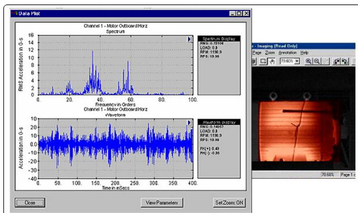
Vibration analysis brings a broad range of tools including Fast Fourier Transforms, time waveform, phase analysis, stress wave analysis, and others to diagnose equipment condition.
