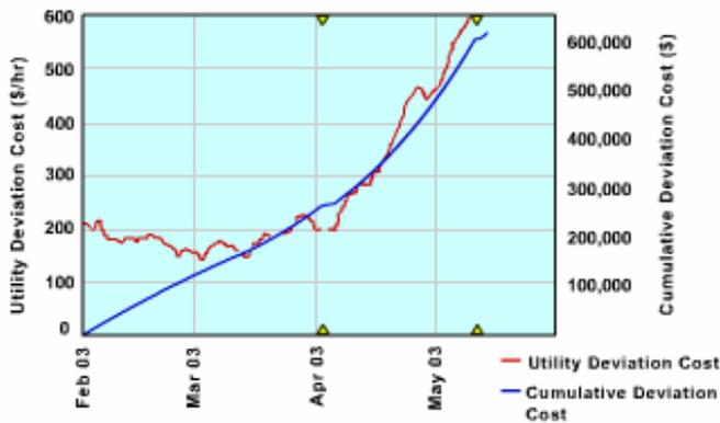
This graph shows the **hourly** and **cumulative** cost of reduced efficiency. This allows a run-versus-maintain decision to be made based on cost and profitability.
