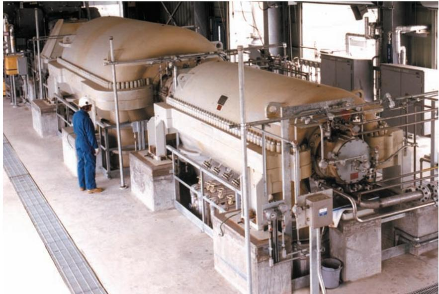
*The cracked gas compressor is an ethylene plant's most critical asset.
