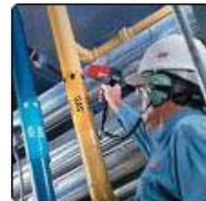
**Motor current analysis** can detect power problems that reduce motor life through excess loads or power imbalance that stresses parts of the motor.
