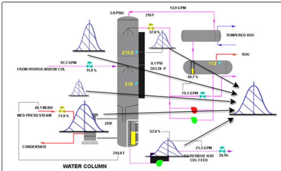
In a typical operating unit, variability can be found in many different places. Every control loop can be a source for variability.
