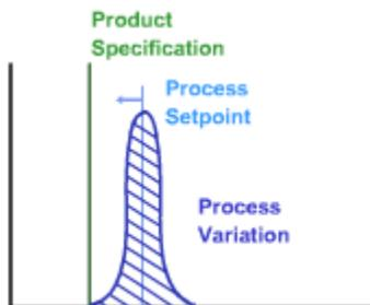
Once the loops are tuned, the setpoints can be moved closer to the product specification once again. This will reduce possible scrap or feedstock costs, and improve throughput.
