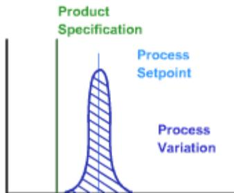
In the beginning, if loops are tuned, variability is at a minimum, and the setpoint is close to the product specification.
