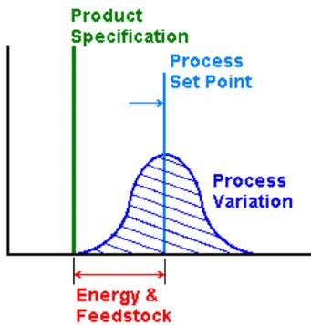
One solution is to move the setpoint farther from process specification. This, however, might increase energy and feedstock costs and cause throughput and efficiency loss.
