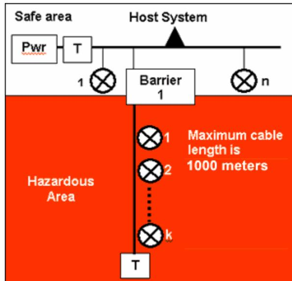
In this example, there are  $n$  devices in the safe area and  $k$  devices in the hazardous area. The maximum number of devices on a segment is 32. Experience demonstrates that up to 16 devices are acceptable. So  $k+n$  must be less than or equal to 32 or 16, depending on the type of devices being used.
