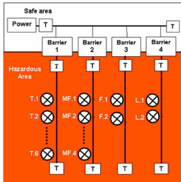
As shown, one possible solution is to put each of the four processes on a separate barrier.
