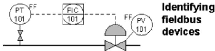
You can also use a different line style for the connection between fieldbus devices.
