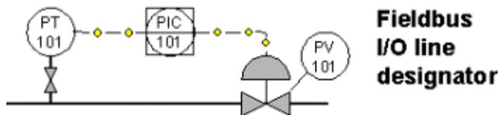
**Indicate where control resides,** especially if it's in a field device. You can do this by placing a small "FF" next to the PID or other function block. Then, to indicate where the control block resides, place the function block symbol next to the field device that will execute control.
