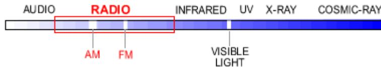
Radio waves used in wireless communications are part of the electromagnetic frequency spectrum.
