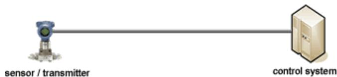
Process-automation communications have traditionally used wired connections between the source and the receiver.
