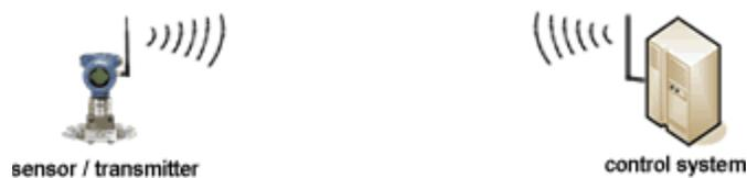
A wireless connection uses radio waves as the communication medium.
