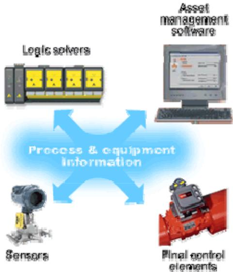
A smart SIS takes advantage of information flow throughout the complete safety loop. This flow includes not only traditional measurement and control data, but additional information on equipment and process health.
