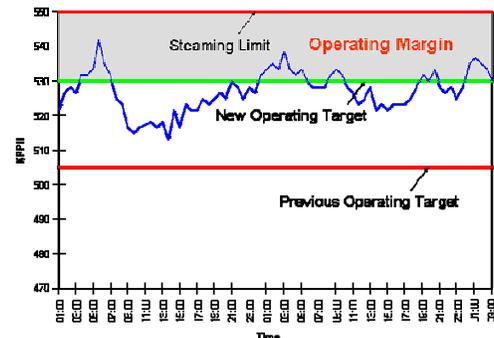
The figures above show how SmartProcess® Recovery is used to reduce variability in boiler process parameters such that additional liquor throughput can be accomplished.
