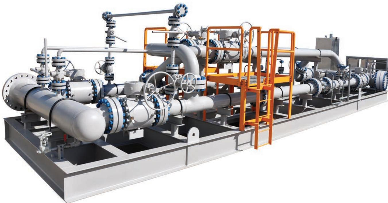
*Figure 3: Completed meter on a skid, ready for installation. The tubes are factory aligned meter-to-tube, conditioner plates, and approach/discharge spools are concentrically aligned, and bolts are drawn up in sequence. All flowmeters, thermowells, analyzers, and other equipment have been installed, wired and calibrated.*
