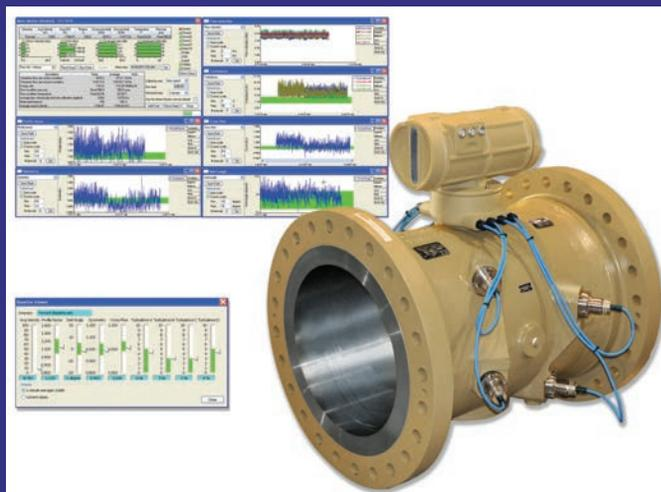
*Figure 4: MeterLink™, Daniel ultrasonic flow meter diagnostic software, enables easy access to expert flow analysis, alerts operators of abnormal flow profiles, and suggests corrective actions. Baseline Viewer™ provides immediate visual indication that the meter is operating within desired ranges.*
