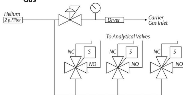
**Figure 2 - Flow Path with Nitrogen on Air Actuation Gas and the Pneumatic Shut-off Valve Installed**
