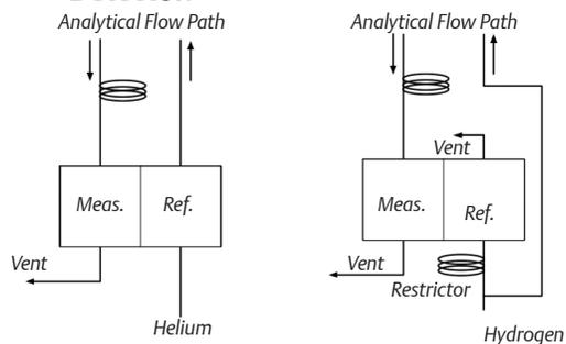
To avoid the rapid degradation of the detector, the hydrogen carrier is routed to the reference detector through a restrictor and the hydrogen supply to the analytical flow path is routed around the detector. The restrictor is matched to the restriction of flow of the analytical flow path to ensure the flow across the reference detector is similar to measure detector.
