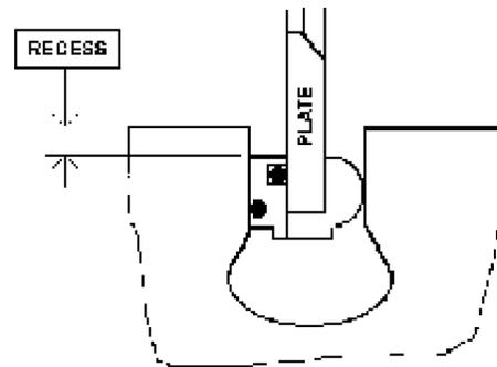
Figure 3: Seal Protrusion
