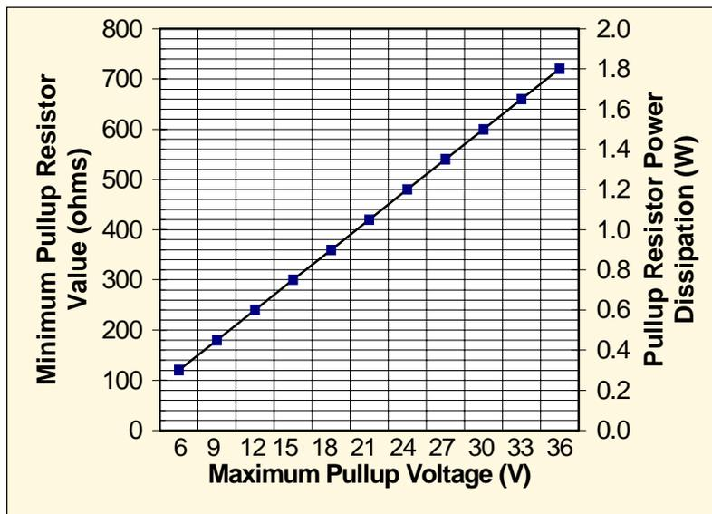
**Figure 3: Pullup Resistor Parameters**
