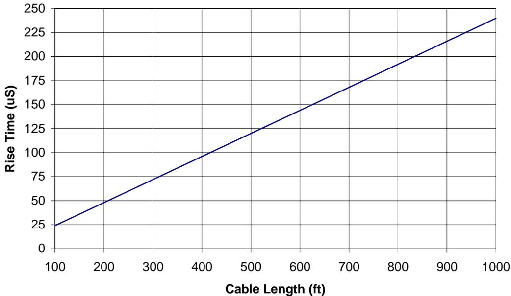
**Figure 4: Rise Time vs. Cable Length (2K Pullup)**
