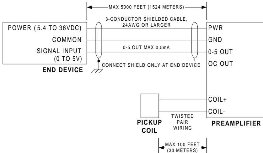
**Figure 1: 0-5V Output Wiring**
