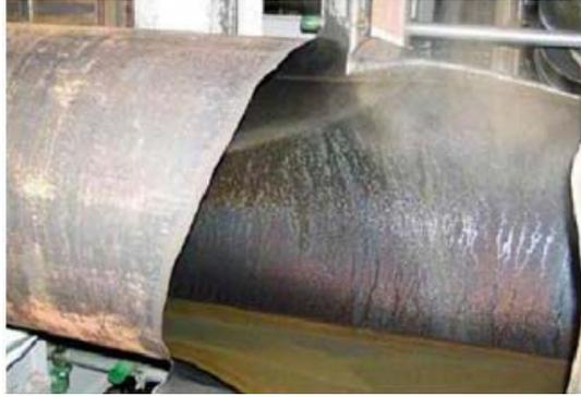
Condensate can also cause rust and corrosion, especially in carbon steel steam pipes, condensate recovery systems and tracing lines. With a properly functioning steam trap, condensate is removed so the steam stays dry. Little air and water is present in the system and rust is less likely to form.
