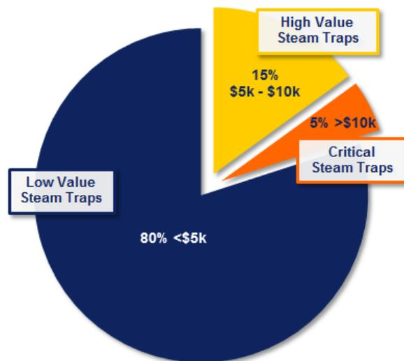
[Figure 7](#) shows about 80% of steam traps in a typical plant do not have nearly the combined financial impact of the other 20% of relatively higher value traps. There are a relatively small number of traps with a very large combined financial impact, and these are referred to as high value steam traps. High value traps are not only those which cause significant steam loss, but also those which can severely and negatively impact plant operation because they:
