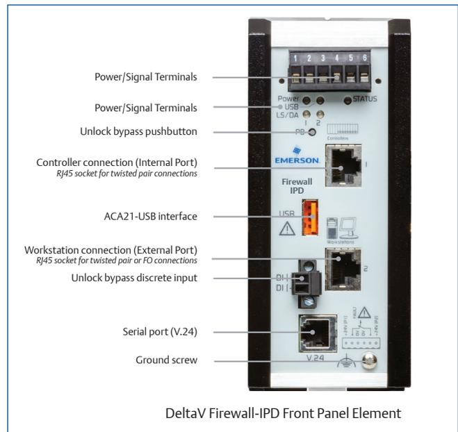
on the secure side of the firewall. CIOCs and controllers should be connected to the same secure side of the same firewall if there is any need to communicate.
