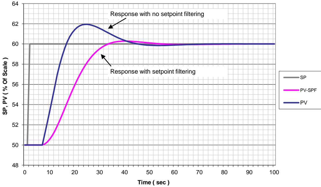
Figure 6. SP filtering
