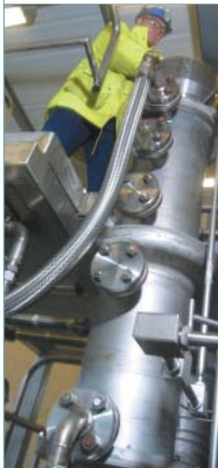
*FIG. 2: Close-in shot of the SCF reactor where pressures of up to 500 bar are maintained.*
