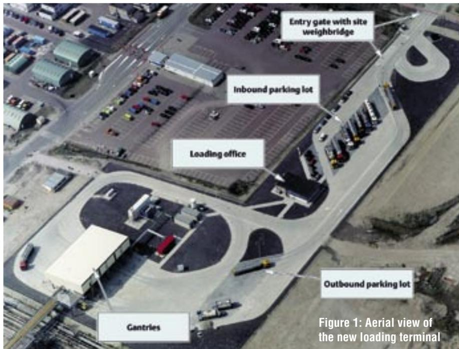
Figure 1: Aerial view of the new loading terminal
