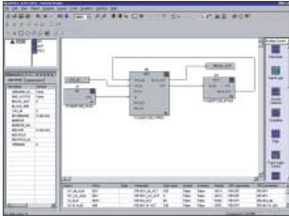
CONFIGURATION SOFTWARE CAN EASE DOCUMENTATION. THIS SCREEN DUMP OF AN IEC 61131.3 FUNCTION BLOCK DIAGRAM-LANGUAGE TEMPERATURE LOOP CONFIGURATION ESSENTIALLY BECOMES A CONTROL LOOP SHEET.
