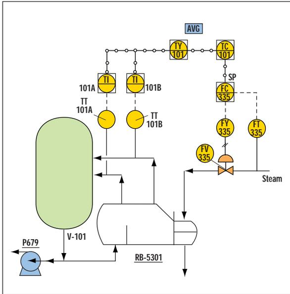
THIS P&ID FOR A HYPOTHETICAL REBOILER ON A DISTILLATION COLUMN IS REFLECTED IN THE FIELDBUS SEGMENT DRAWING OF FIGURE 2. IF A CONTROL STRATEGY USES TT101'S INPUT SELECTOR BLOCK, A REPLACEMENT DEVICE MUST CONTAIN THAT FUNCTIONALITY OR THE BLOCK MUST BE MOVED.
