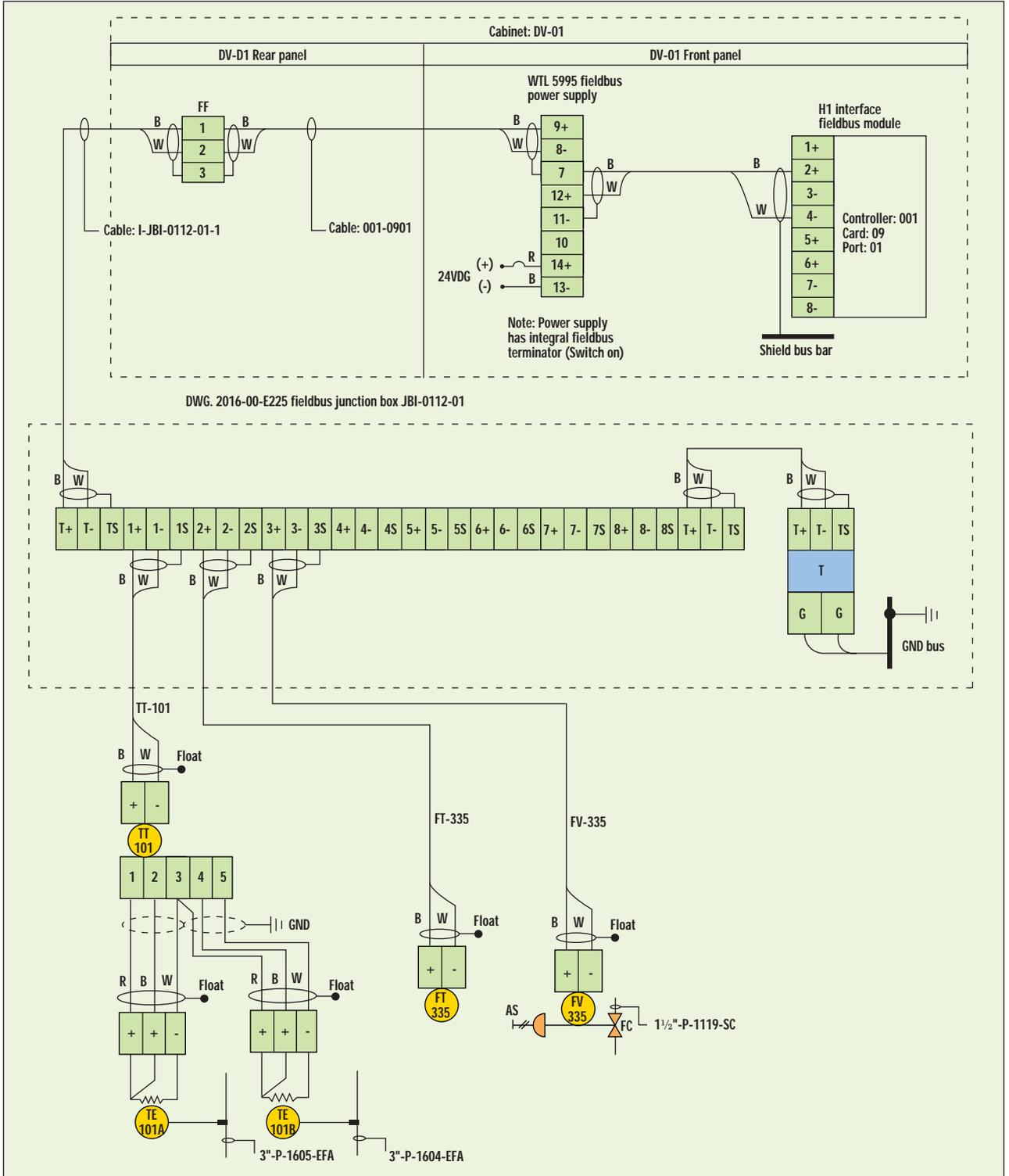
FOUNDATION FIELDBUS SEGMENT DRAWING FOR THE HYPOTHETICAL REBOILER IN FIGURE 1. LIMITING THE SEGMENT DRAWING TO ELECTRICAL DETAILS HELPS AVOID MAKING IT A REPOSITORY FOR SUPERSEDED INFORMATION.
