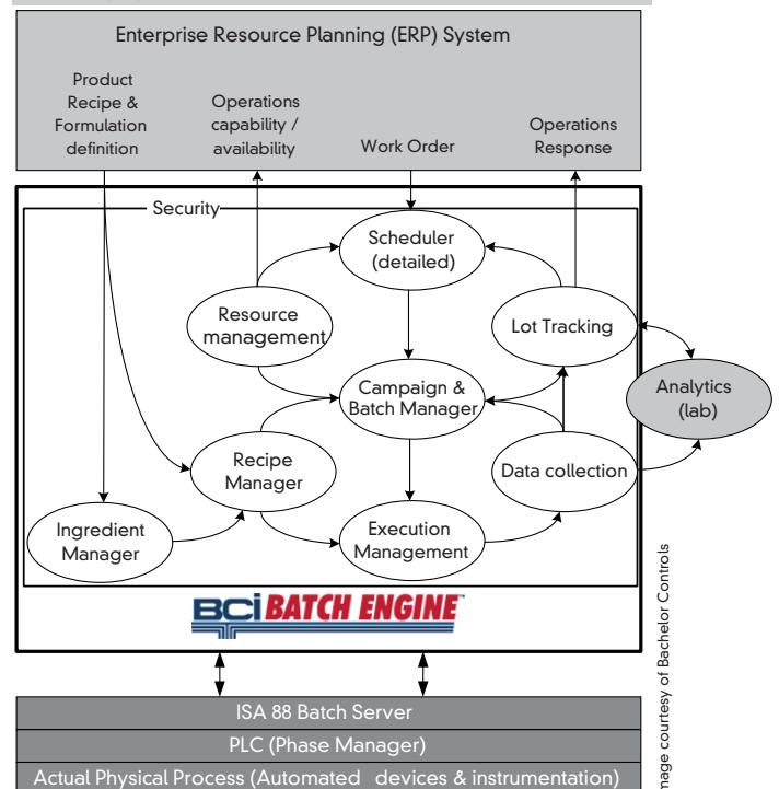
Middleware like the batch engine software shown in this diagram is often used as a transfer point for communications between plant control systems and ERP systems
