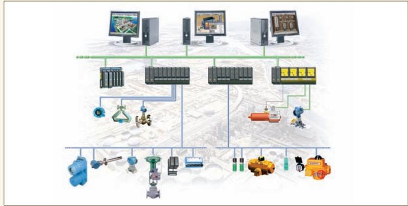
*Integrating safety and process controllers implies sharing a common environment without compromising proper operation of the SIS.*
