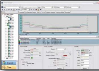
Students and professors can use DeltaV to explore process automation applications and new technologies, to gain new understanding of the behavior of dynamic systems. The DeltaV system can be used in the educational environment to tune traditional PID control, model predictive control, create neural networks, implement fuzzy logic, and perform variability analysis.
