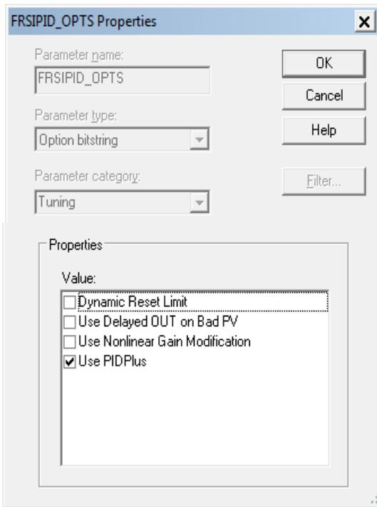
Figure 1 - PIDPlus enabled in FRSIPID\_OPTS for PID block
