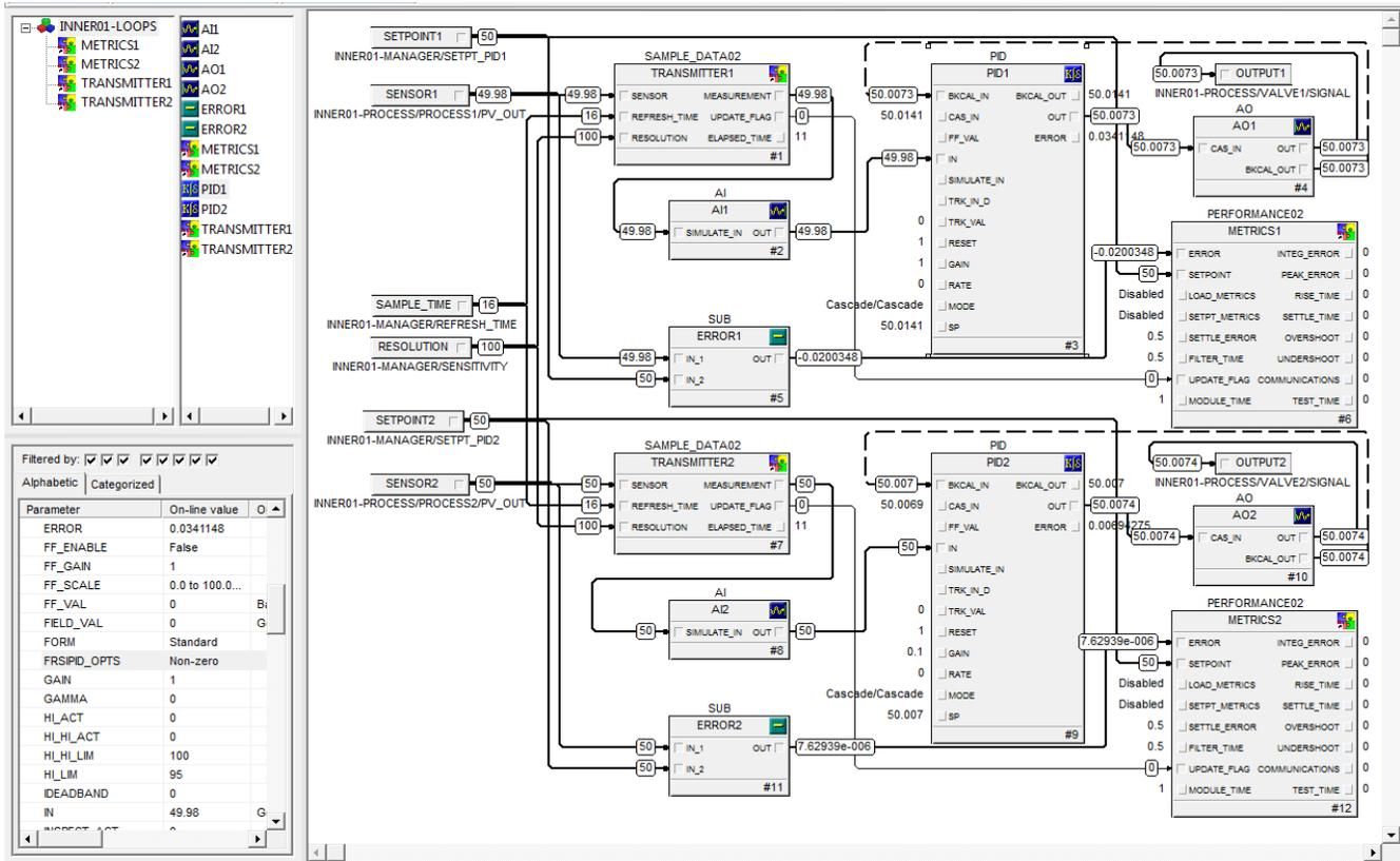
Figure 2 - Test Setup of PID Module
