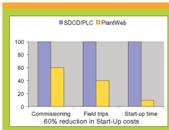
Figure 2: Start up costs comparison (in %) between PlantWeb architecture project and traditional system.
