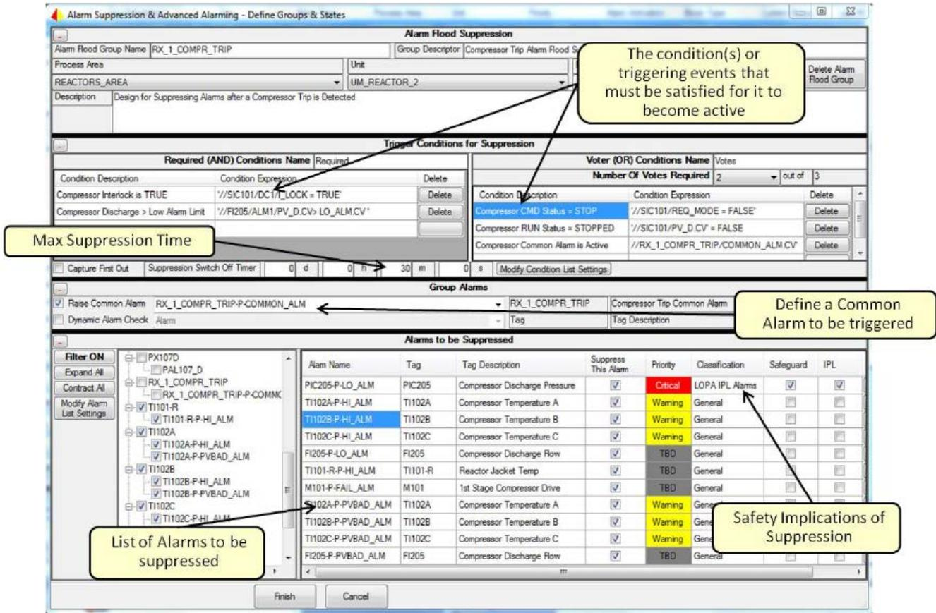
Defining a DeltaV Alarm Flood Suppression Module in SILAlarm.
