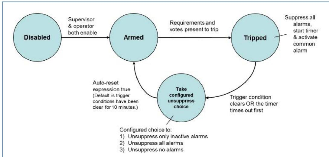
Alarm Flood Suppression module state transition diagram.
