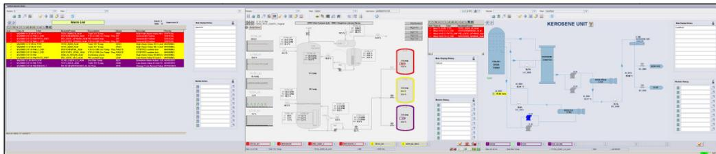
A three-monitor layout puts the working screens in the right two monitors of the workstation.
