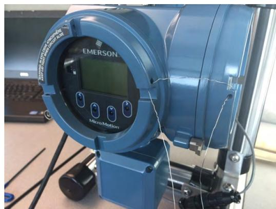
Figure 2. Sealing and Lockout Mechanism
