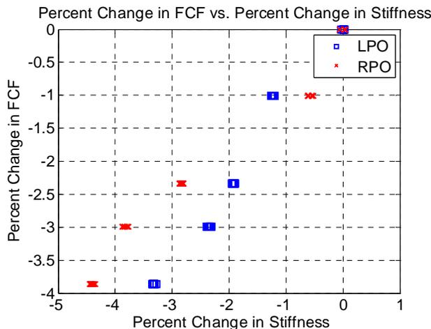
Figure 5. FCF vs Stiffness with Corrosion
