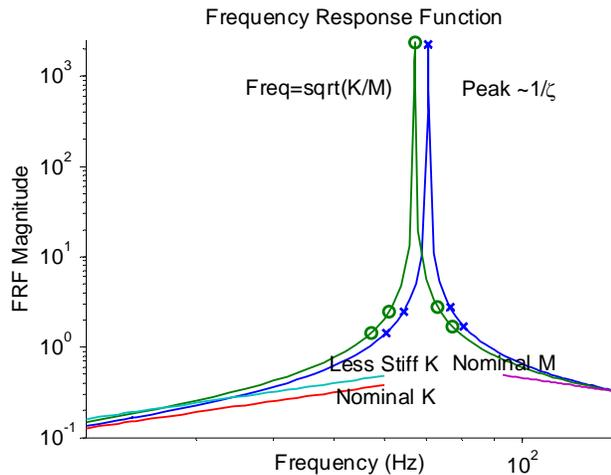
Figure 4. Change in FRF with Stiffness Reduction
