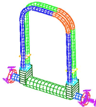
Figure 6. Beam FE Model for Erosion Study
