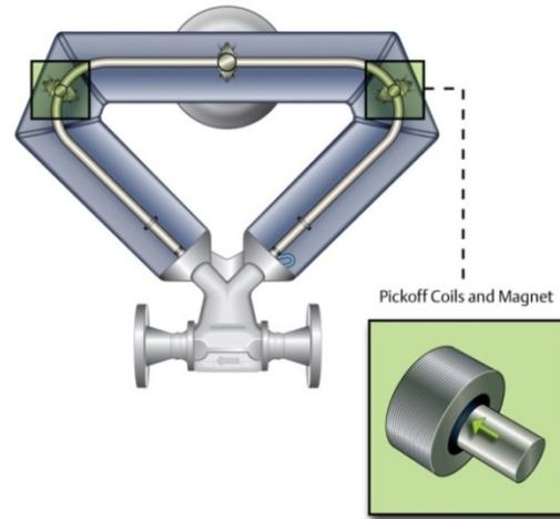
Figure 1. Typical Coriolis Flowmeter
