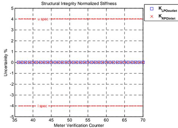
Figure 3. Meter Verification Stability
