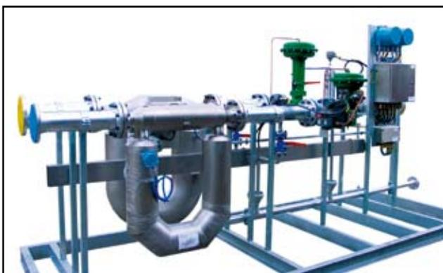
Figure 5. Dual stream blending skid for fuel oil loading.
