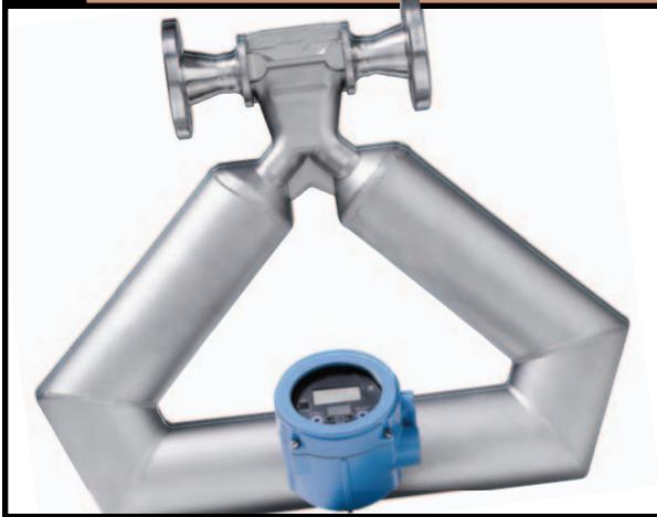
Figure 4. This Coriolis meter employs a series of tones to check for tube stiffness, an indicator of erosion, corrosion and deformation.
