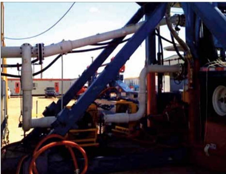
**Top:** Coriolis meters on suction and return sides of the well provide an electronic way of "keeping an eye on the shakers." **Bottom:** This photo shows a side view of an installation on the return flow to the shaker. Return flow installations can be operated on systems with or without rotary heads.
