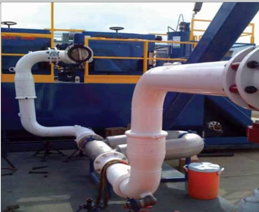
Meters on suction, return sides of well can collect mass/volume flow rate, density in/out info for multiple uses
