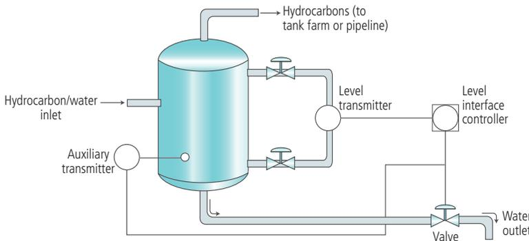
present, because many level systems will miss the rag layer completely and only “realize” the problem after spilling a lot of valuable material. Not only is this wasteful, it is problematic from an environmental standpoint as well, as the waste treatment facility can get overloaded.
