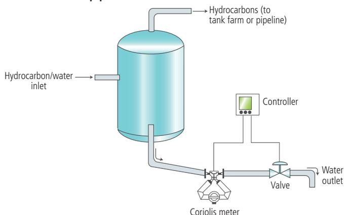
placing the sensing element directly in the waste pipe, we can keep the maximum amount of hydrocarbons in the tank and the maximum amount of water out of the tank.
